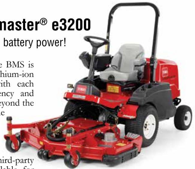
This mower comes with Toro’s InfoCenter™ display with battery charge status, hours, alerts, customizable settings and more. It features the same rugged 60-inch (152 cm) side or rear discharge mowing deck options built with high-strength steel for ultimate durability, and impact bumpers as featured on our popular diesel-powered Groundsmaster models.
